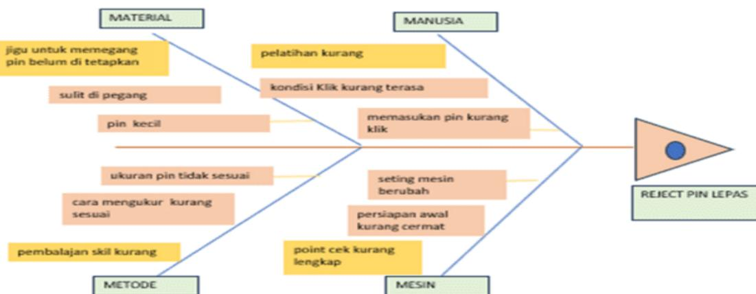
Gambar 4. Diagram Fishbone Reject Pin lepas
