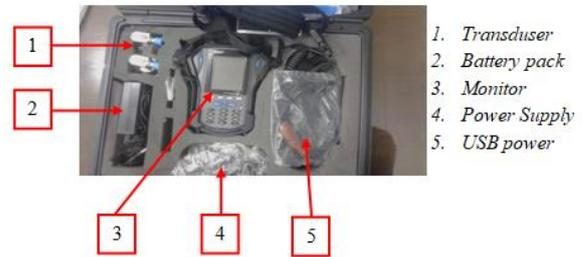
Gambar 2. *Vibration Analyzer SKF Microlog gx Series (Cmx 75)*
